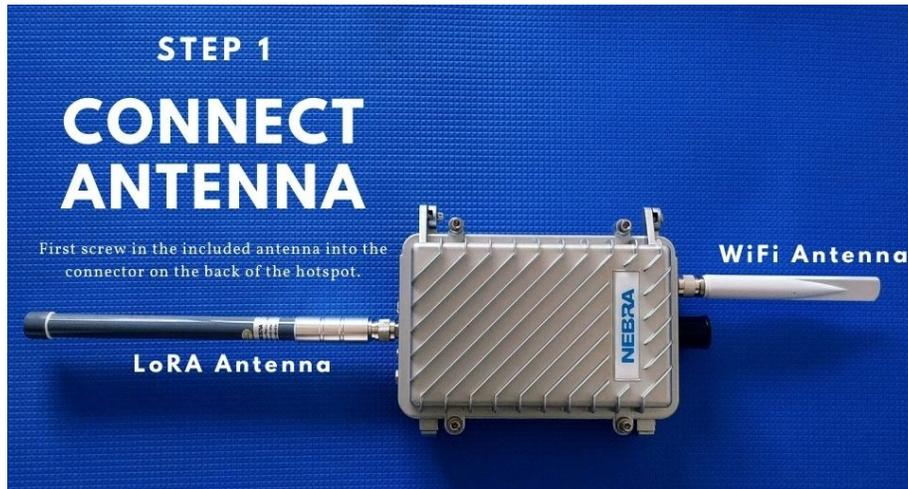
Figure 2: Outdoor Hotspot Antenna
