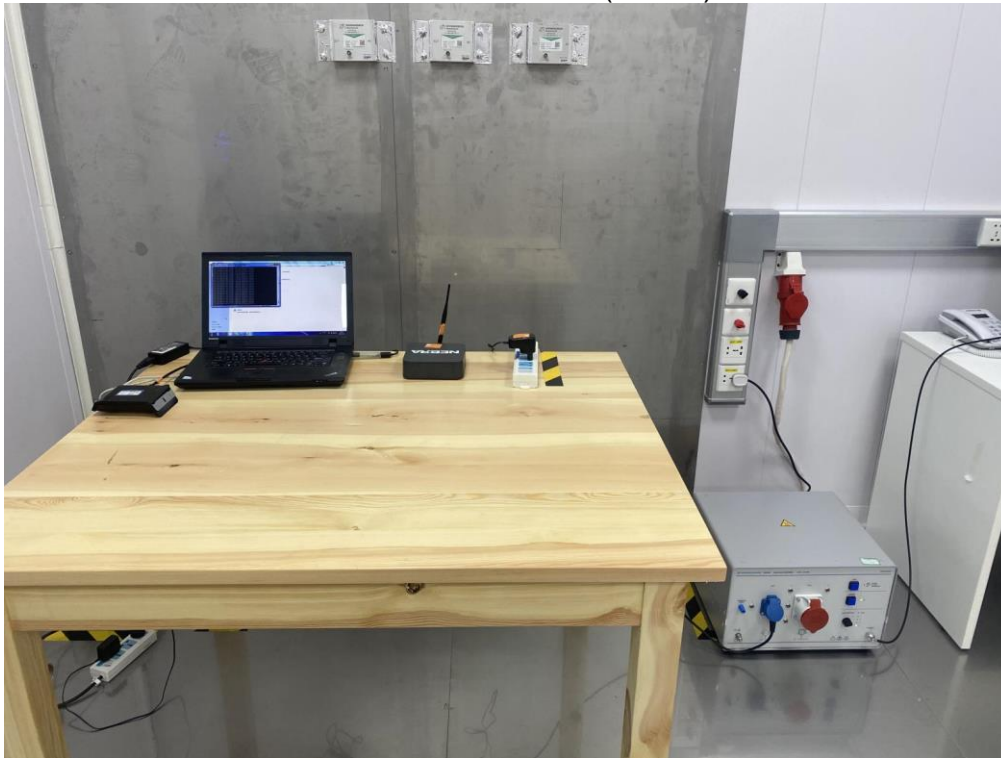
Conducted Emission (for AC)
