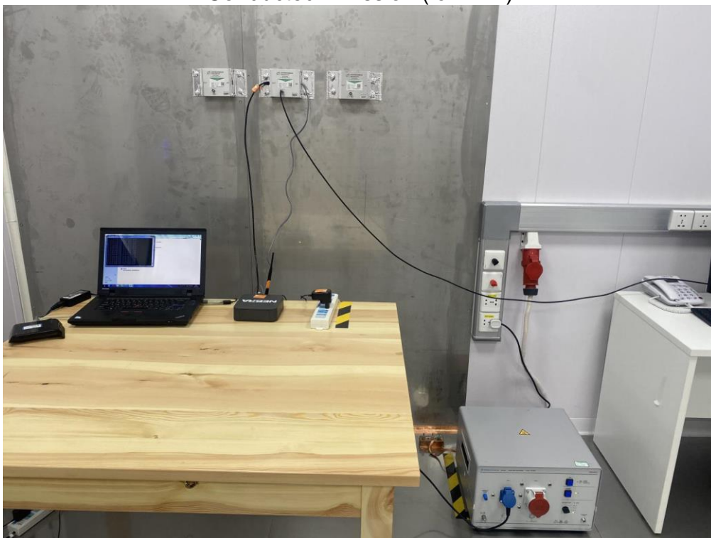
Conducted Emission (for LAN)
